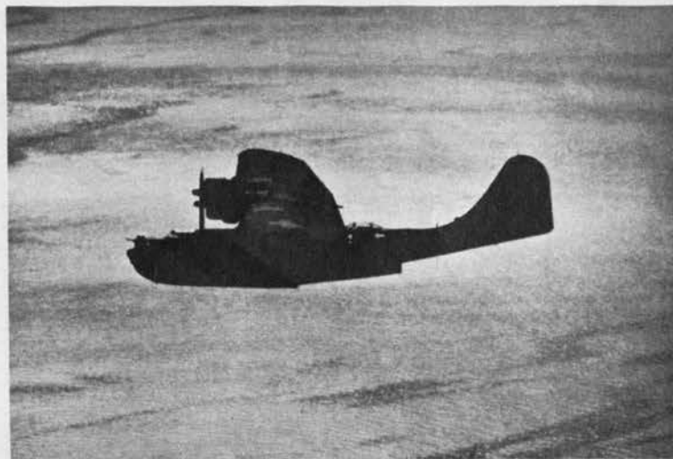
Shallow hull of a patrolling PBV, with its up-swept, smoothly faired fin and rudder, is slung beneath the broad, rectangular wing surface.
